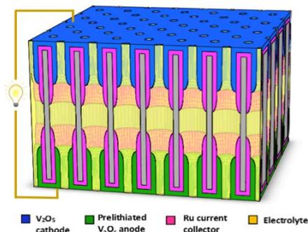
Nanostructured batteries promise to deliver energy at much higher power and with a longer lifetime than conventional technology. With rational design and controlled fabrication, researchers have demonstrated nanopore batteries that can quickly charge and discharge over many cycles.
