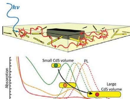
Luminescent solar concentrators based on tunable CdSe/CdS nanorods enable concentration of both direct and diffuse sunlight onto highly efficient micro-silicon solar cells, demonstrating a practical path to operation in the high-concentration regime.
